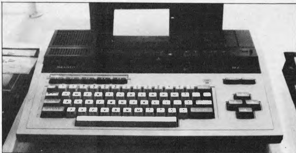
This is Sharp's MZ-700 with the optional four-colour plotter and cassette deck. It's software-compatible with the MZ-80K/A machines, has 64k RAM as standard and colour output to a TV set.
